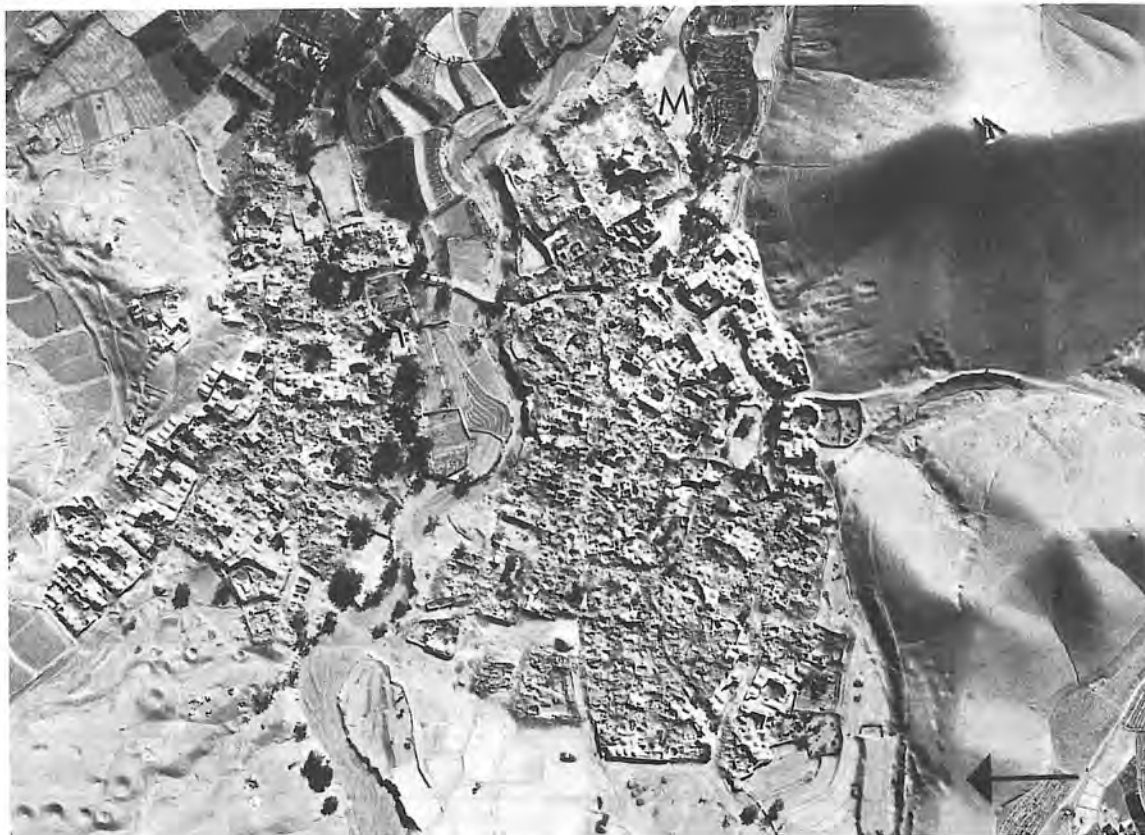
Plate 2(a). Damage to adobe houses built in clusters: Aerial view of the village of Kariskh (9 kilometres west of Dasht-i Biyaz) taken after the earthquake of 31 August 1968. Notice that with the exception of a few houses southwest of the mosque (M), the village was totally destroyed (80% of the houses collapsed killing 20% of the people, see Ambraseys & Tchalenko 1973).
