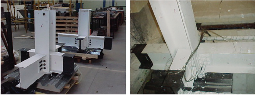
Figure 3.4 Unprotected secondary beam with coatback at the connection (Li et al., 2017, Dai et al., 2009).
