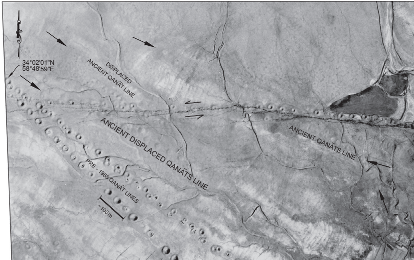
PLATE 13.4 Aerial photograph of the 31 September 1968 M_w 7.1 Dasht-e Bayāz earthquake surface rupture in the area north-northwest of Miām and east of Dasht-e Bayāz village (see Figure 13.1 for the location). Left-lateral offset of the stream beds can be seen. Two lines of NW–SE-trending younger qanāts (traditional ancient Iranian underground aqueduct system; indicated by their circular access shafts) are located to the left (west). A set of older abandoned NW–SE trending qanāt lines can be seen to the northeast and north of the younger qanāt lines. Additional old, abandoned east–west trending qanāt lines are also present in the vicinity of the Dasht-e Bayāz fault trend. The older qanāts were damaged and displaced by historical earthquakes along the fault (dates unknown). Courtesy of the National Cartographic Center of the Imperial Government of Iran, October 1968.
