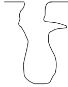
Figure 6.19 Irregular grout distribution
