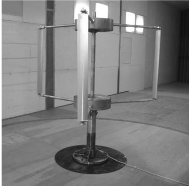
Figure 17.3 Vertical axis wind turbine in a wind tunnel.
