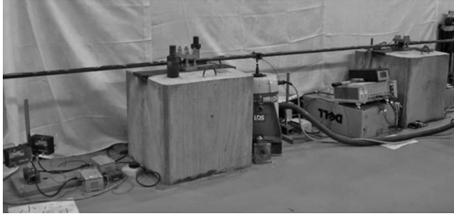
Figure 8.7 Experimental arrangement of overhanging beam.
