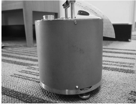
Figure 3.5 Photograph of a seismometer. (From https://en.wikipedia.org/wiki/File:CMG-40T_Triaxial_Broadband_Seismometer.JPG .)
