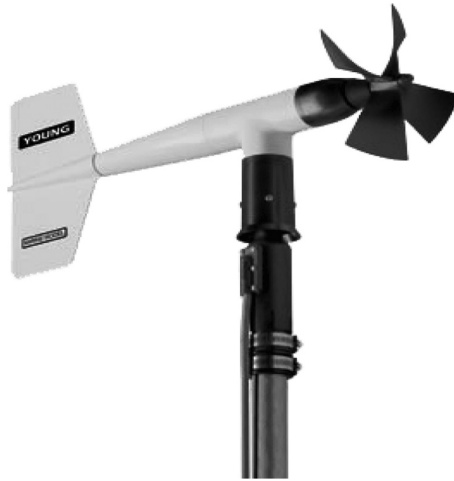
Figure 3.1 Propeller anemometer. (From http://www.junyangchina.com/ProductShow.asp?ID=182. )
