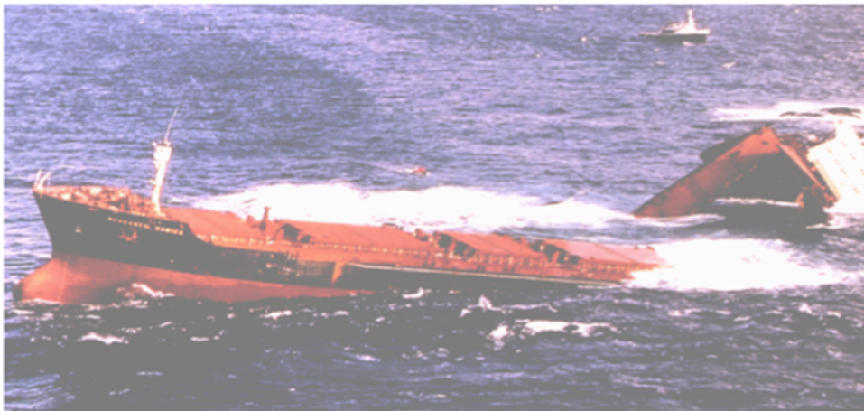
Figure 8.4 Collapse of ship's hull girder: (a) during unloading of cargo at port; (b) at sea.
