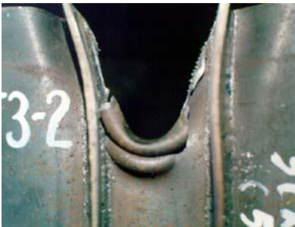
Figure 10.28 A concertina tearing.
