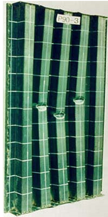
Figure 7.2 A typical collapse pattern of the corrugated panel under lateral pressure (Paik et al. 1997).
