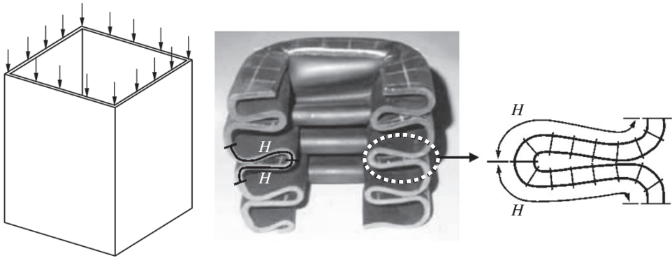
Figure 12.6 Crushing behavior of a plated structure and the necessary size of the finite elements.
