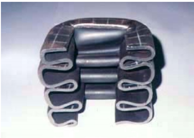
Figure 10.17 A plated structure crushed under axial compressive loads and cut at its midsection.
