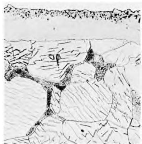
Fig. 5 Nitrided case and diffusion zone produced by cyanide-cyanate liquid nitriding. The characteristic needle structure is seen only after a 300 °C (570 °F) aging treatment. Depth of compound zone about 0.01 mm
