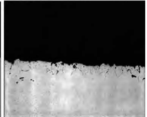
Fig. 5 Surface layer after carburizing to a case depth of 0.7 mm (0.03 in.). Material is SAE 5115; scale is 1000:1.
