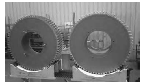
Fig. 2 Gear parts for a wind turbine coated with stop-off paint (Condursal 0118) prior to case hardening
