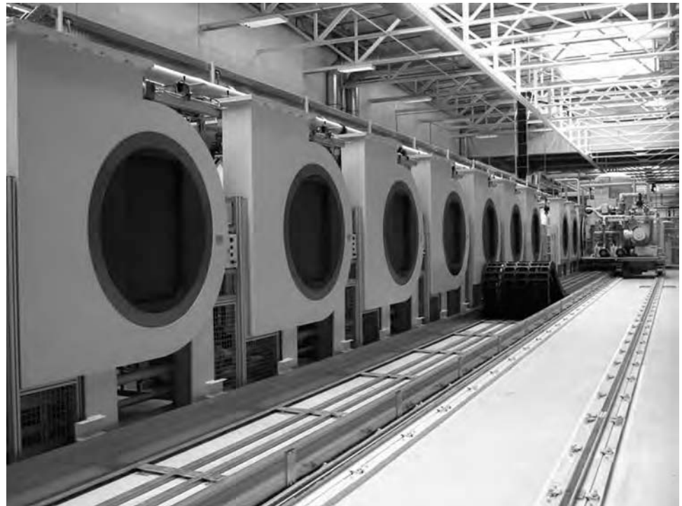
Fig. 8 Multichamber system for low-pressure carburizing process in mass production. ModulTherm (ALD Vacuum Technologies) with ten treatment chambers
