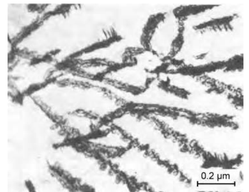
Fig. 13 Transmission electron micrograph showing cementite precipitated on dislocations in an 0.08C-0.63Mn steel aged 115 h at 97 °C (207 °F). Courtesy of J.E. Indacochea (Ref 21)
