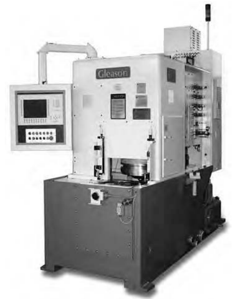
Fig. 2 Modern version of the Gleason 529 quenching machine. Courtesy of The Gleason Works, Rochester, NY
