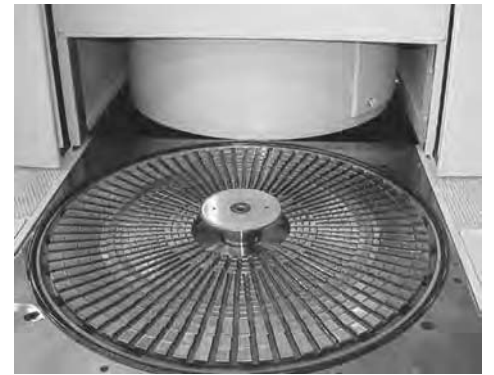
Fig. 5 Lower die assembly of a quenching machine in the "out" position. Note the spring-loaded center expander cone and the individual slotted rings. Courtesy of The Gleason Works, Rochester, NY
