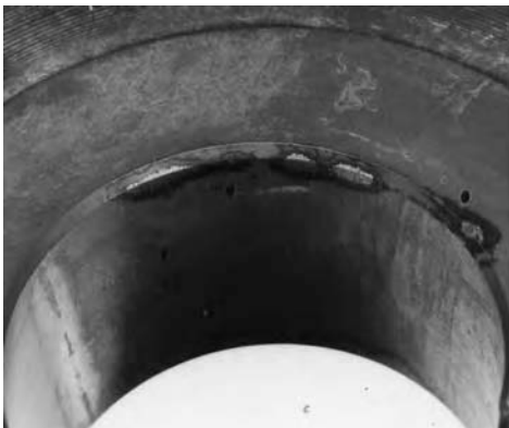
Fig. 21 Example of oxidation and succeeding corrosion observed at the upper edge of a ring coated by high-temperature borax baths. No carbide coatings on spotty bright areas surrounded with black areas
