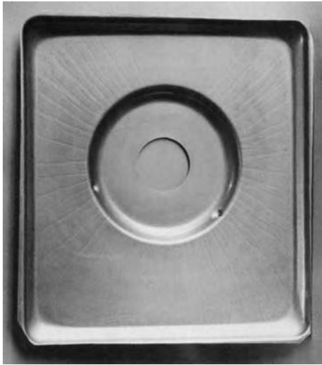
Fig. 15 Stretcher-strain marks (Lüders bands) on the surface of a range component after forming. Original magnification: 0.25x
