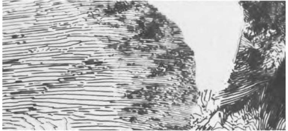
Fig. 32 Pearlite that was formed isothermally in steel by partial transformation at 700 °C (1290 °F) and by further partial transformation at 674 °C (1245 °F). The pearlite at left was formed when the specimen was at the higher temperature and is coarser than the pearlite at center, which was formed when the specimen was at the lower temperature. Composition of steel: 0.87 C, 0.44 Mn, 0.17 Si, 0.21 Cr, 0.39 Ni
