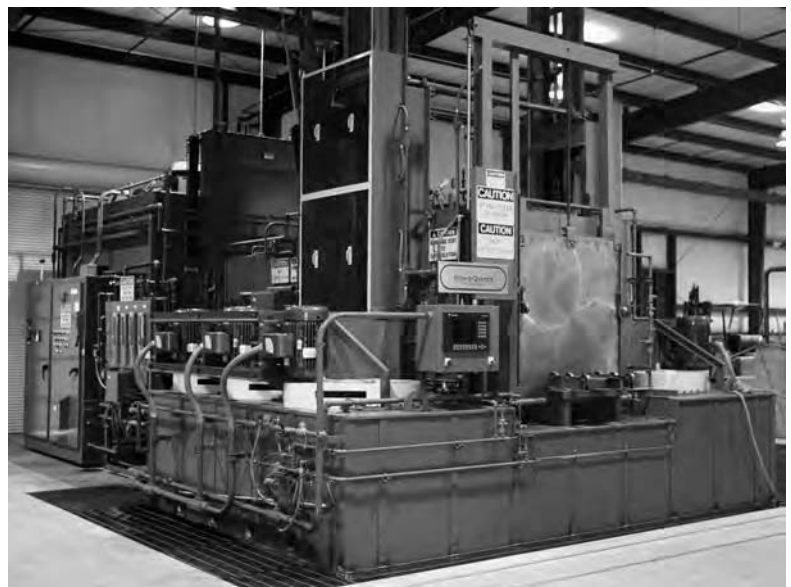
Fig. 16 Integral quench atmosphere furnace equipped with intensive quenching water tank. Source: Reprinted from Ref 3 with permission of ASTM International
