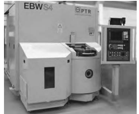
Fig. 19 Load-lock cycle facility for hardening. Chamber volume: 0.04 m 3 ; beam parameters: 60 kV, 6 kW. Courtesy of PTR
