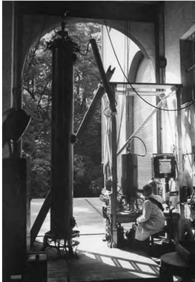
Fig. 1 Bernhard Berghaus in 1947 at his institute with a pit furnace developed for plasma nitriding of gun barrels.
