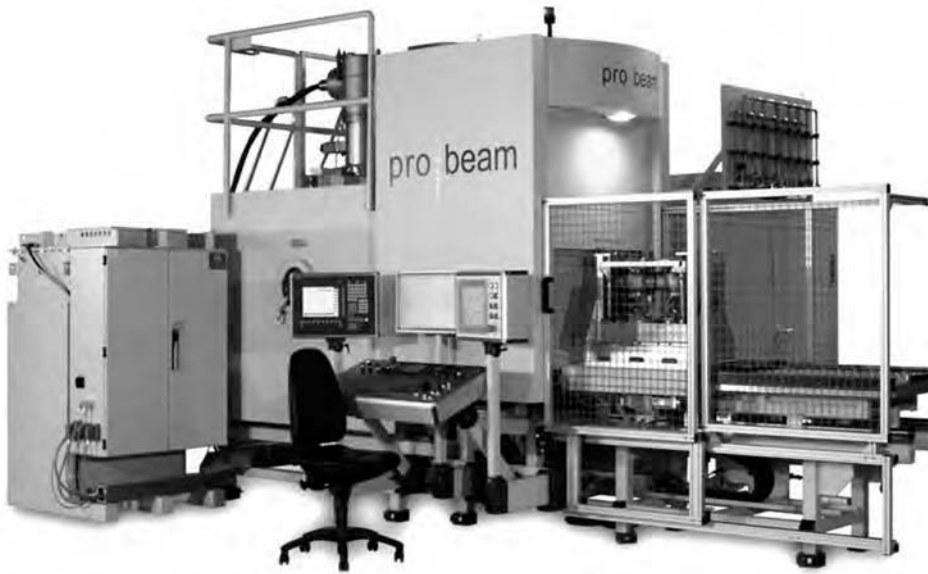
Fig. 20 Load-lock shuttle facility for hardening and welding. Chamber volume: 2 m 3 (71 ft 3 ); beam parameters: 60 kV, 10 kW. Courtesy of pro-beam
