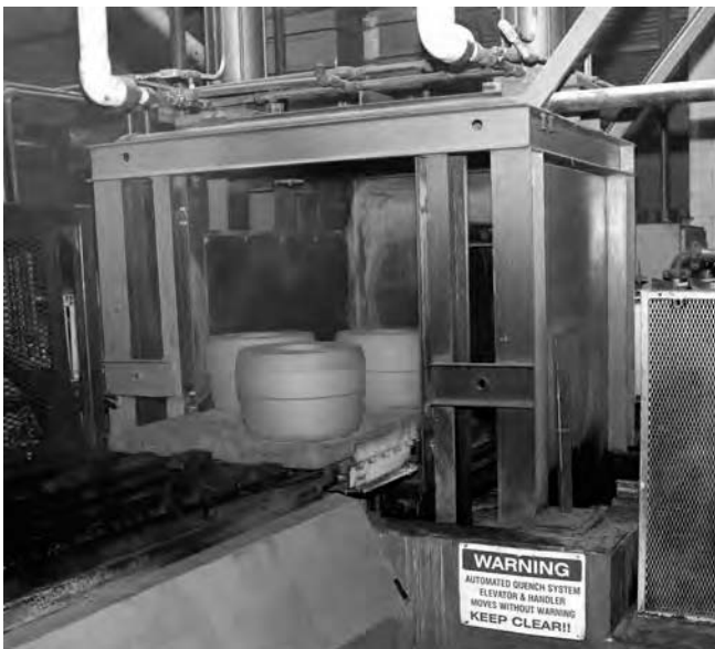
Fig. 15 Batch-type intensive quenching (IQ) system with stand-alone IQ water tank. Courtesy, Akron Steel Heat Treating Co.
