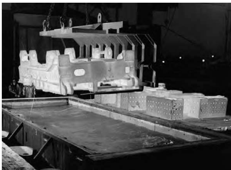
Fig. 101 Photo of austenitized steel casting just prior to immersion into the quench oil. Source: Ref 254
