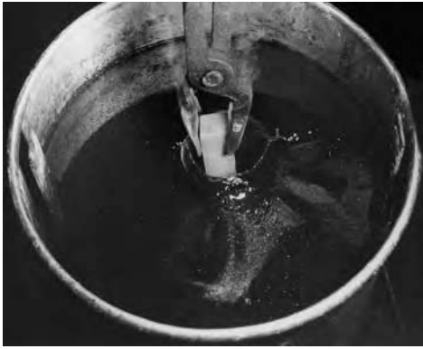
Fig. 45 Quenching a 25 mm (1 in.) square bar of austenitized steel into room-temperature water. This clearly illustrates immediate vapor blanket formation. This photo was taken only 0.0001 s after immersion. Courtesy of E.J. Cox, Pittsburgh Commercial Heat Treating Co.
