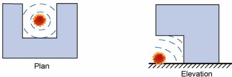
Figure 6-3 Schematics showing the effect of building shape on air-blast impacts
