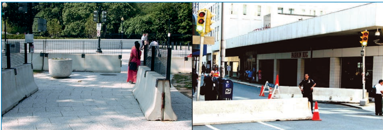
Figure 4-29: Jersey barriers: pedestrian disruption at the White House (left) and on a D.C. Street (right).
