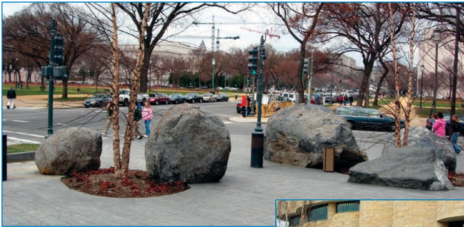
Figure 4-27: Selected rocks and custom bollards as barriers: scale and placement provide nonintrusive security.
