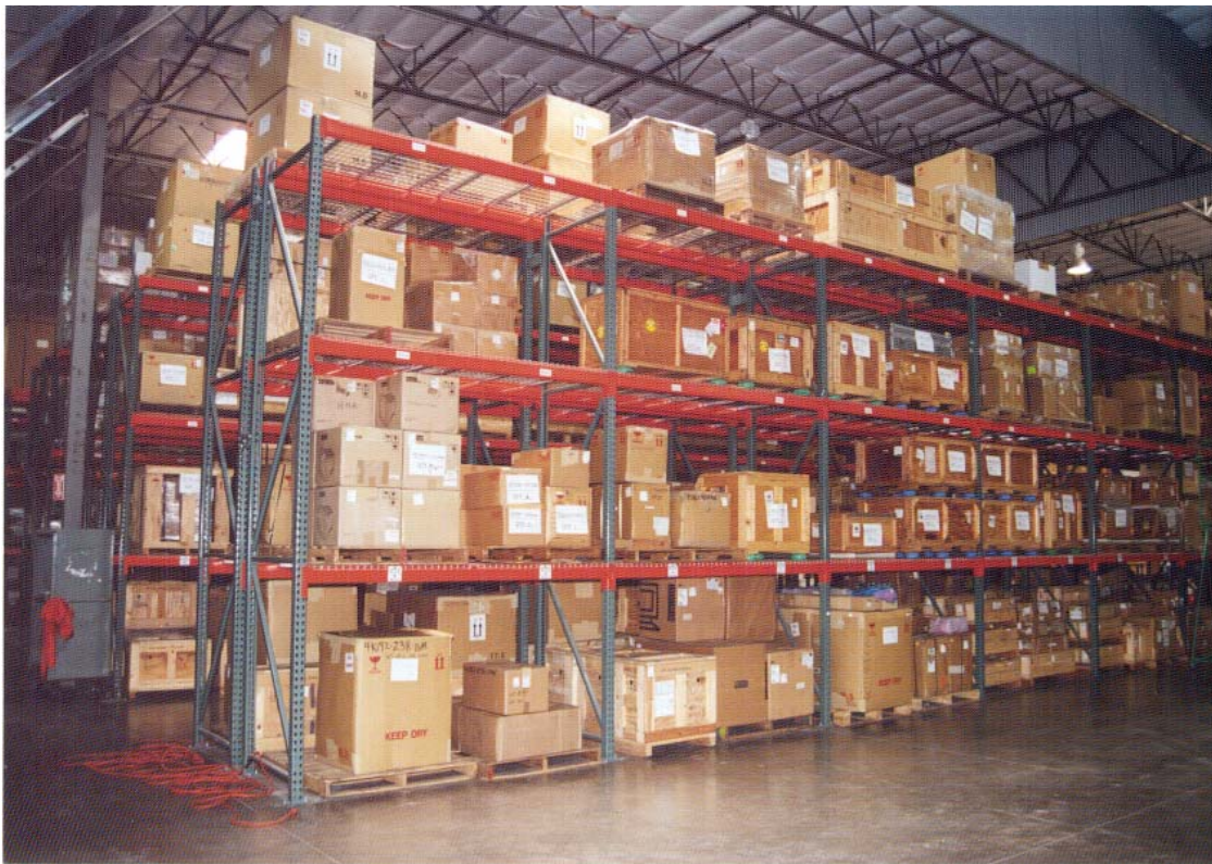
Figure 1-1 Typical steel single selective pallet storage rack.
