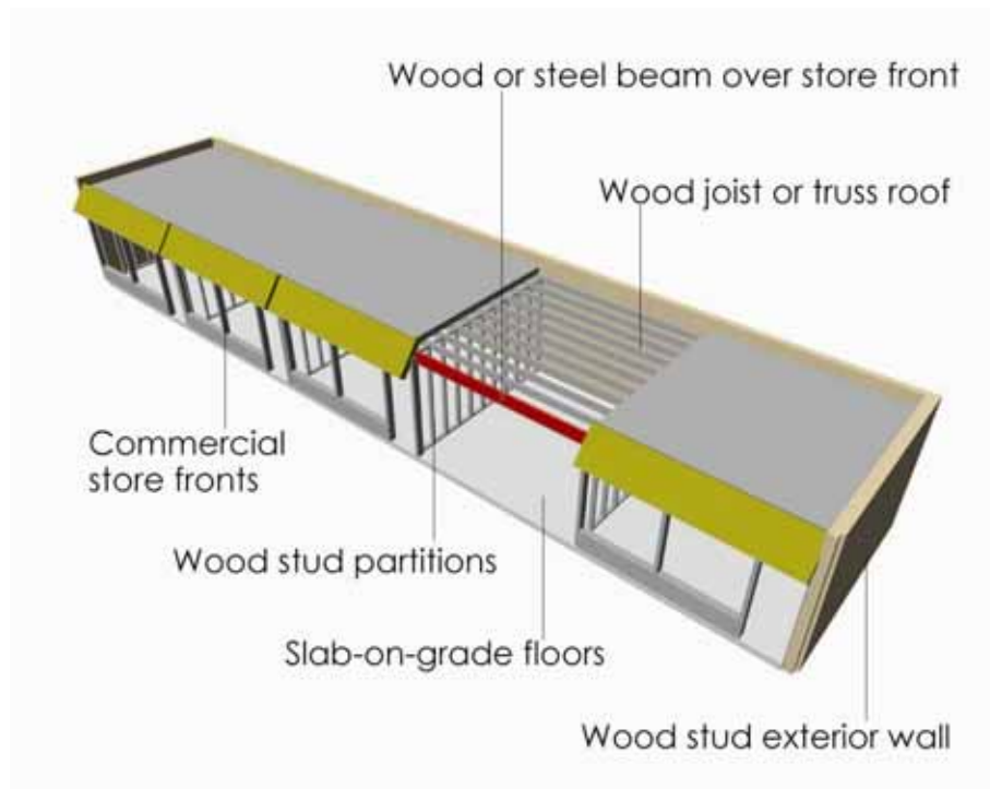
Figure 7.1-1: Building Type W2: Woodframes, Commercial and Industrial
