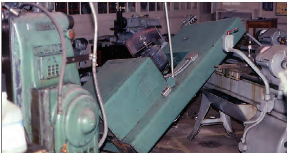
Figure 4-9: Fallen shop equipment, Coalinga, CA, 1983
