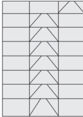
Figure 8-9 Example of an in-plane discontinuity irregularity.
