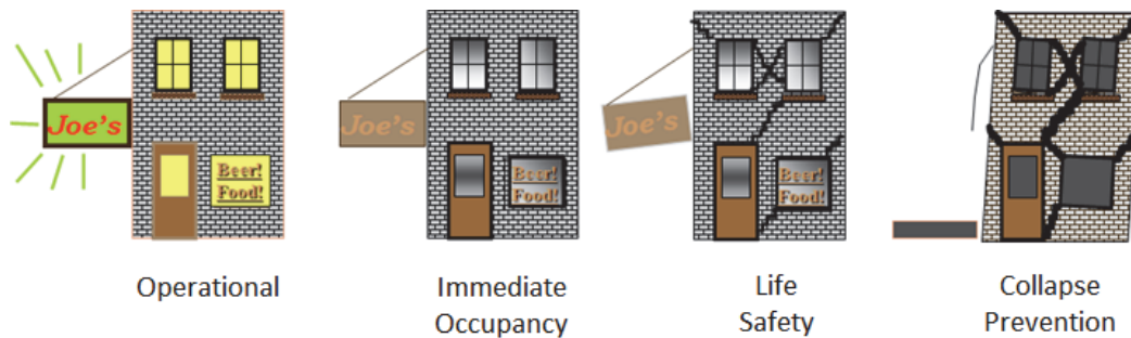
Figure 10-1 Standard ASCE/SEI 41 performance levels.
