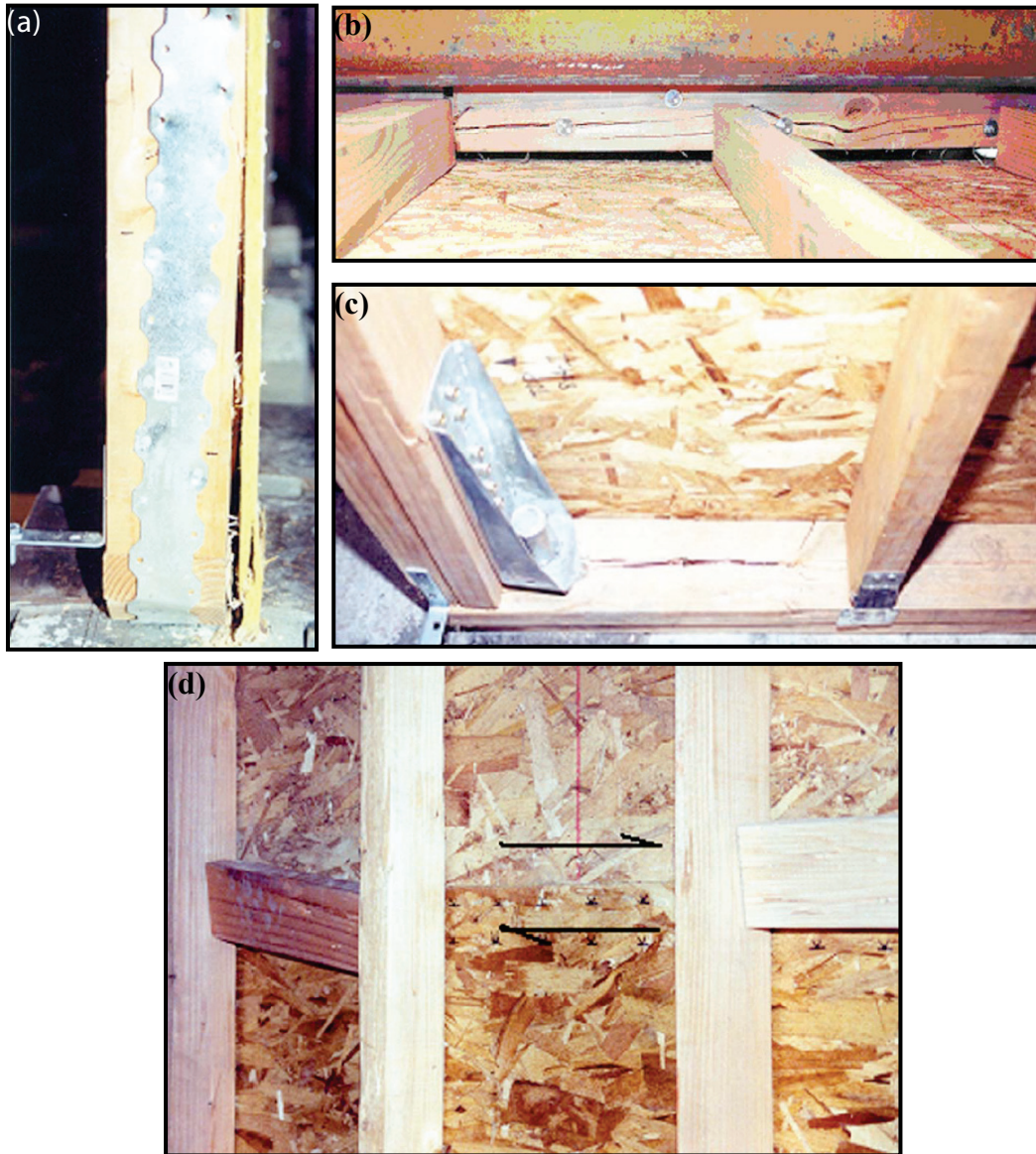
Figure D-1 Failure modes of stapled wood shear wall test specimens showing: (a) staple withdrawal for wall number 4-C; (b) staple and splitting of top plate for wall number 12-A; (c) anchor rod failure and splitting of sill plate for wall number 8-C; and (d) staple shear and blocking failure for wall number 8-B (from Talbot et al., 2009).
