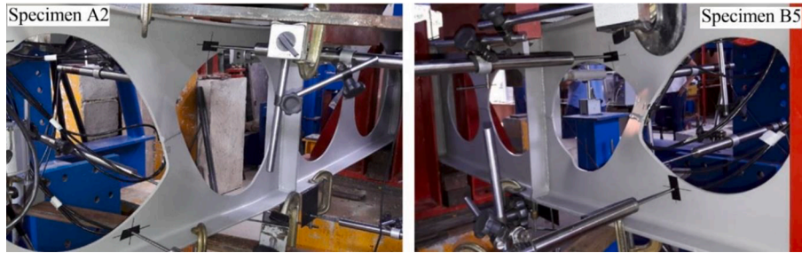
Fig. 16. Web-post buckling of steel cellular beams under shear action [563].
