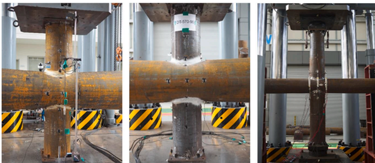
Fig. 37. CHS X-joints tested by Kim et al. [366].
