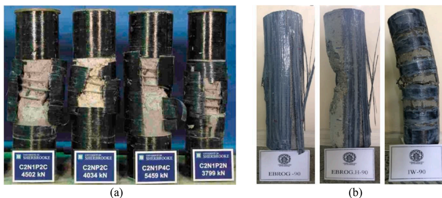
Fig. 21. FRP-strengthened RC columns under (a) concentric load [568] and (b) eccentric load [569].
