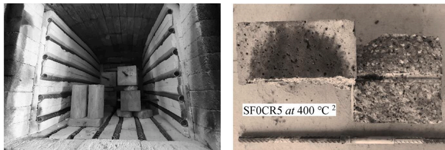
Fig. 23. Bond post-fire bond behaviour of steel bar in steel fibre concrete [178].
