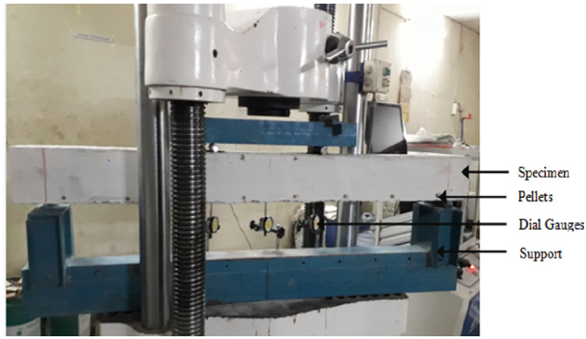
Fig. 3. Details of test setup and Instrumentation.
